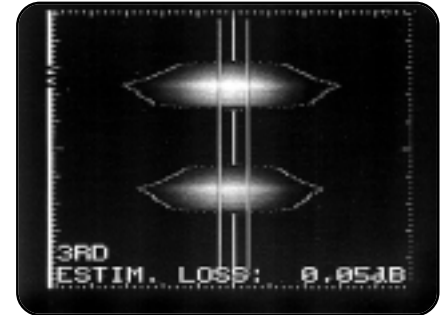
Hot image of depressed cladding fibers
