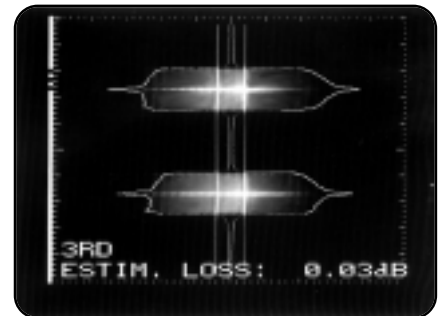
Hot image of erbium + single mode fibers
